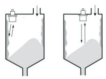
The transducer should not be mounted too close to the tank wall, the build-up on the tank wall cause false echoes.
