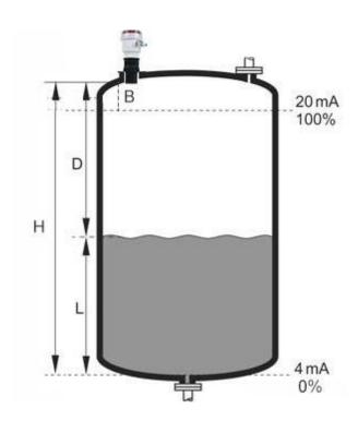
The principle of operation of the ultrasonic sensor system is to use the ultrasonic pulses which are transmitted by the transducer to the surface to be monitored and are reflected back to the transducer, the time period between transmission and reception of the sound pulses is directly proportional to the distance between the transducer and surface The latest microcomputer technology and the proven processing software select the level echo from
