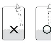
Keep transducer perpendicular to liquid.
