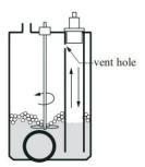
As is illustrated by the figure on the right, the transducer should be mounted on the top of guide tube to prevent the false echoes from turbulence and foam. The guide tube should come with a vent hole at top of the tube to allow the liquid vapor go out of the tube.
